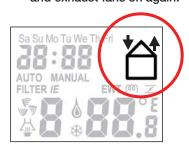
Bear in mind that switching off the supply or exhaust fan will temporarily immobilize your balanced ventilation system.
