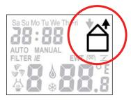
This mode can be used when the windows are open during the summer. In that case, fresh air is not supplied via the supply fan, but through the open windows.
