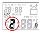
In addition to showing the programmed ventilation setting, the CC Ease panel also displays whether a temporary control system (such as a  $CO_2$  sensor or a bathroom switch) is overriding the ventilation setting.
