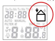
3. Press " Three times to switch the supply and exhaust fans on again.
