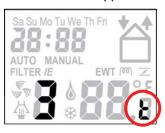
Once the programmed time delay is complete, the ComfoAir automatically switches back to the previous ventilation setting.
